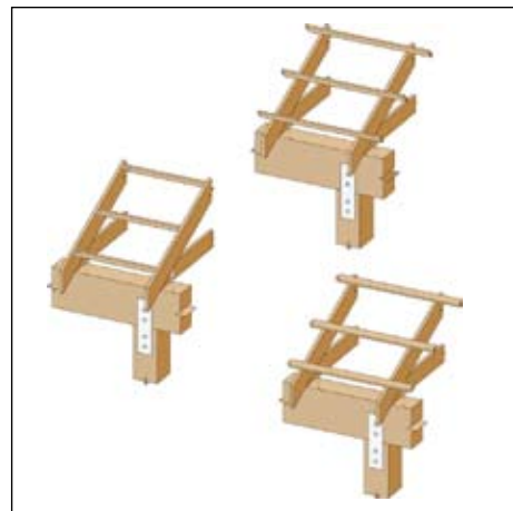
Figure 34. Post to Glu-lam or SCL header and header to truss connection.
